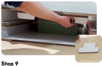
Secure the tabs into place on the inside of the column by inserting the stoppers into the tab slots.
